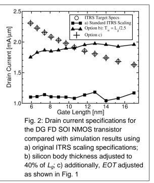
In the 2011 ITRS bulk NMOS was specified for channel lengths down to 14 nm, and SG FD SOI NMOS down to 11.7. For these values the drain current of both architectures was simulated to be rather similar to that of the DG FD SOI NMOS.
