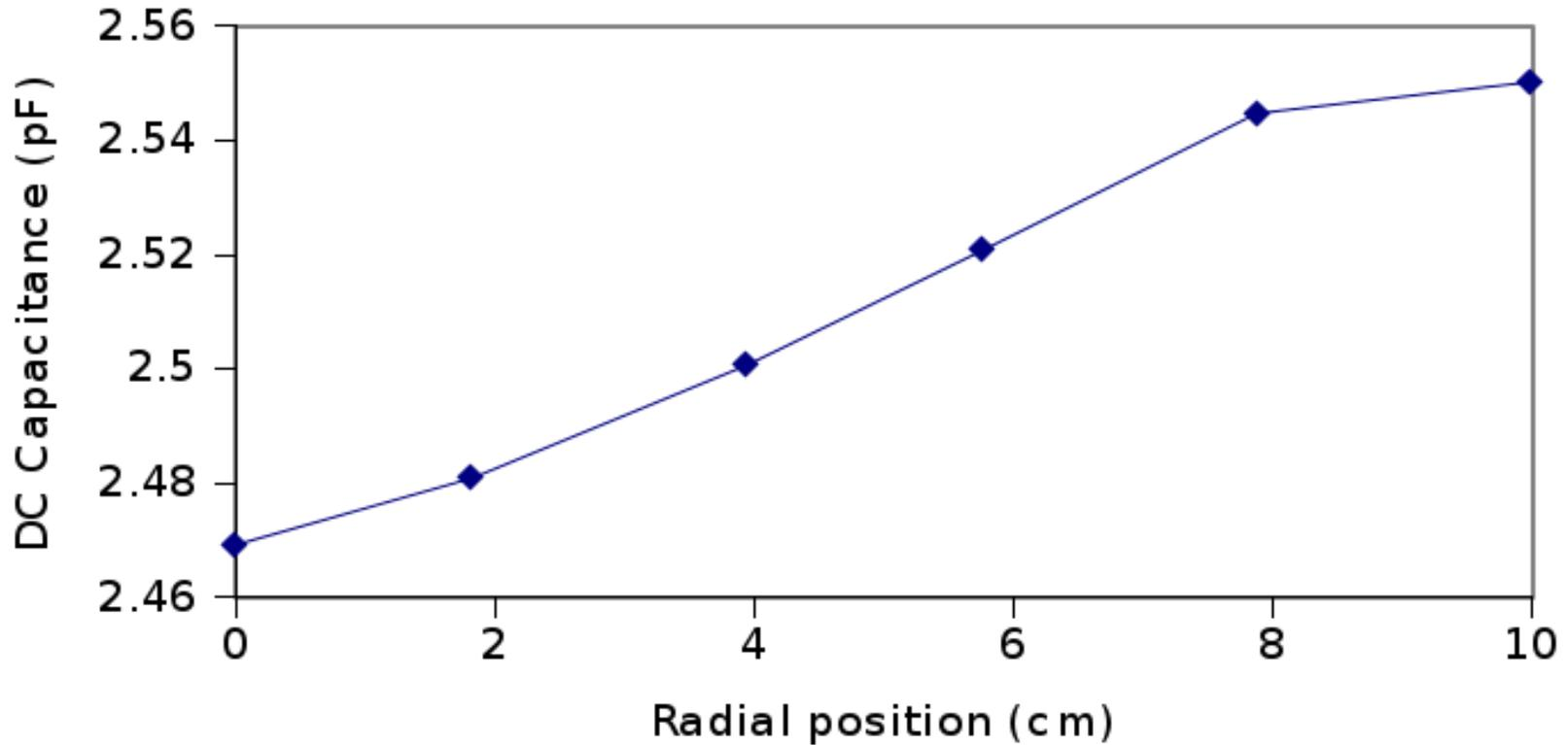
Simulated variation (COMSOL) of DC capacitance between different positions of the TSV structure on the wafer
