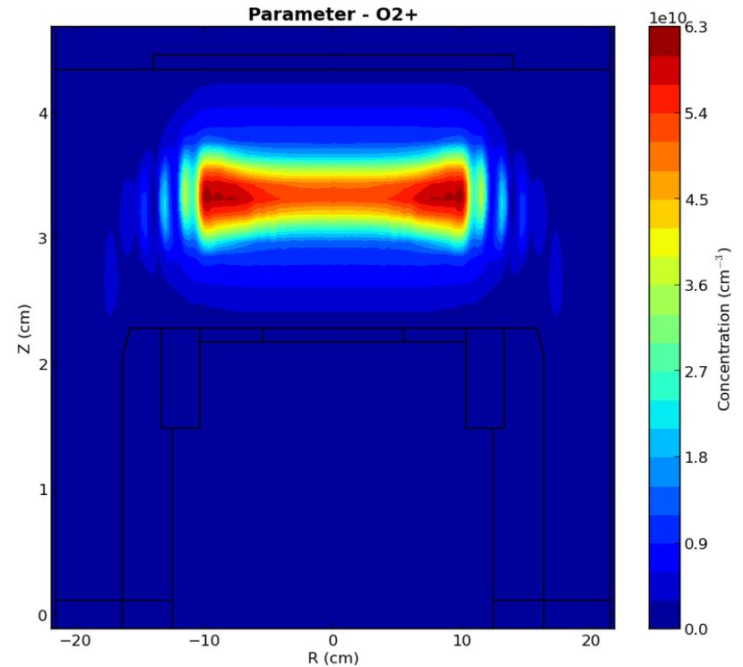
Example for concentration of neutrals (O) and ions (dominant ion species is  $\text{O}_2^+$ ) in a CCP reactor (figure aspect ratio is scaled)
