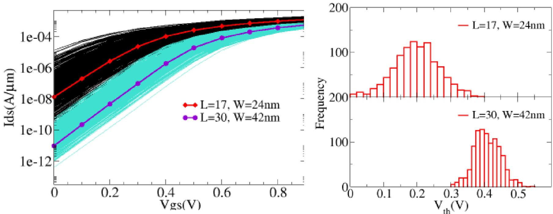
SPICE simulated IV-characteristics of 2 corner transistors due to GV in L and W resulting from combined lithography step and statistical variability due to RDD, LER and MGG.
