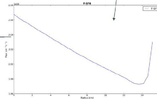
SF6 distribution on wafer surface at one sequence loop
