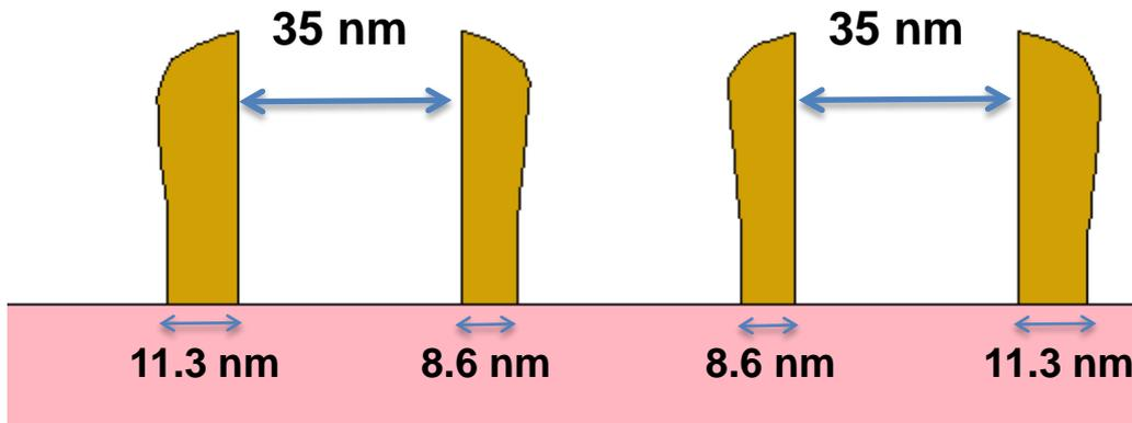
Simulation for **nominal CD (35 nm)** of carbon lines
