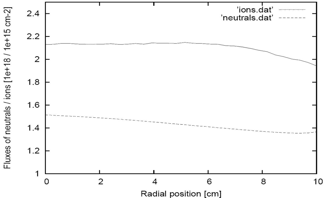
Example for flux at wafer vs. radial position for neutrals (O) and ions (dominant ion species is  $\text{O}_2^+$ ) in a CCP reactor
