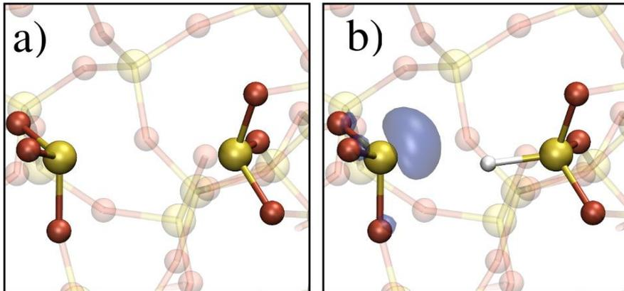
a) Atomic structure of the **oxygen vacancy** which is the precursor to the hydrogen bridge
