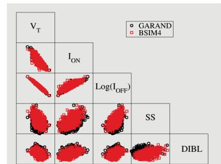
Simulation examples: Gate length vs. focus and dose variations in optical lithography (IISB - left); atomistic device simulation with variability sources *RDD*, *LER* and *MGG* (GU - middle); scatterplots of figures of merit obtained from statistical models and GARAND (GSS - right)
