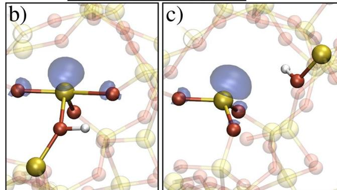
Atomic configuration and spin density of the two hydrogen induced defect configurations and their precursor:
