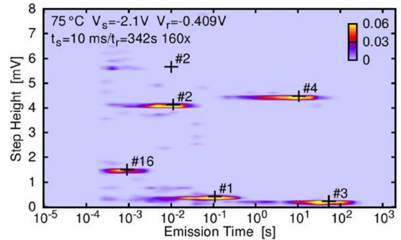
Calculated defect parameters give good agreement with the capture and emission rate dependence on voltage and temperature
