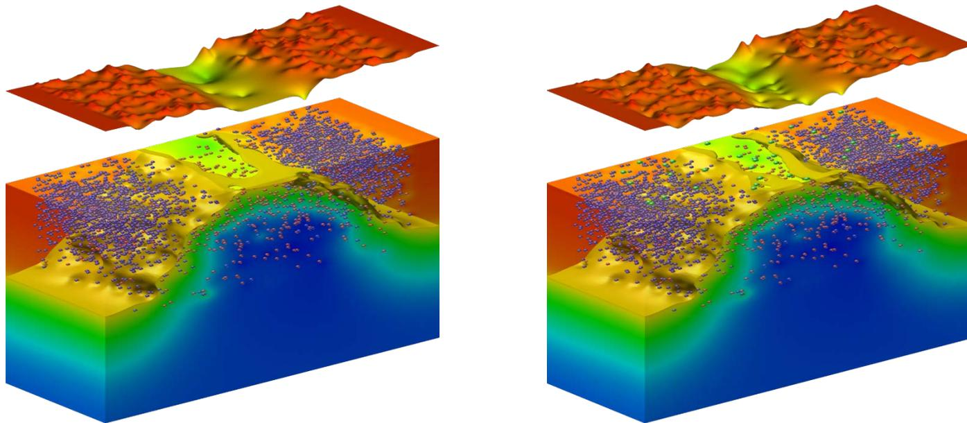
Left: Simulation of a 45 nm technology transistor in the presence of discrete dopant, line edge roughness and polysilicon gate granularity. Right: Simulation of the same transistor subject to degradation. By chance two holes are trapped in the vicinity of the percolation path. From GU / GSS
